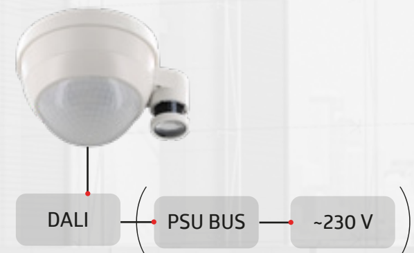
DALI detectors can either be BUS-powered or they have to be supplied with 230 V. In the latter case, the BUS power supply (PSU BUS) is usually already integrated.
