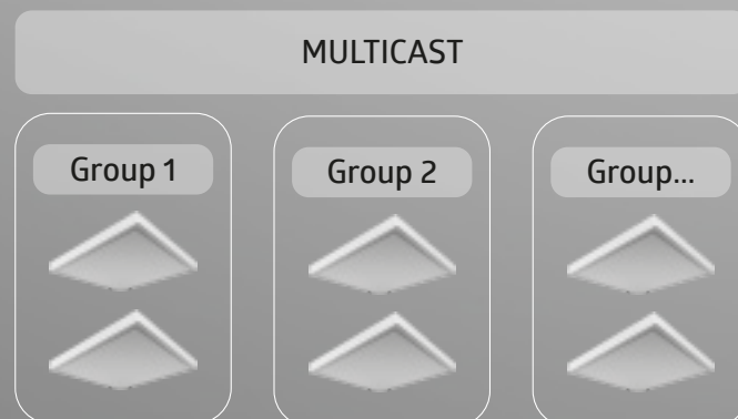
With a multicast telegram, up to 16 groups with different properties can be defined.
