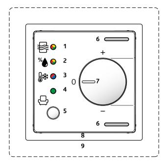
The traffic light indicator (1) on the device can be used to display the air quality. The colour red stands for poor air quality, yellow for medium air quality and green for good air quality. The limit values for red and yellow can be set and a hysteresis can be defined.
