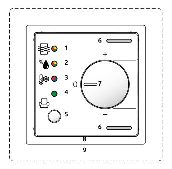
On the housing of the device there is a control knob (**Potentiometer 7**) with which the adjustment can be changed manually. The set value can be adjusted within the limits of the positive and negative offset either via the communication object in steps or by means of the rotary control. The "Set value Reset" communication object can be used to reset the device to the values specified in the ETS.
