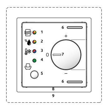
On the housing of the device is a control knob (potentiometer, 7) with which the adjustment can be changed manually. The set value can be adjusted within the limits of the positive and negative offset either via the communication object in steps or by means of the rotary control. The communication object "Set value reset" can be used to reset the device to the values specified in the ETS.
