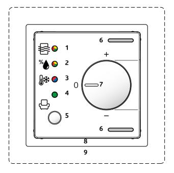
On the housing of the device there is a control knob (potentiometer, 7) with which the adjustment can be changed manually. The set value adjustment allows to define an offset for the set value (positive and negative). The communication object "Set value reset" can be used to reset the device to the values specified in the ETS. In addition, the value can be specified as an absolute value (in %).
