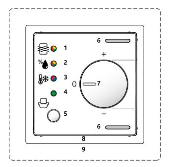
The comfort extension allows the comfort temperature to be kept for a selected period in the event of an unscheduled event. This is done either via the communication object or the pushbutton (5) on the device. The activation of the comfort extension is indicated by the green LED (4).
